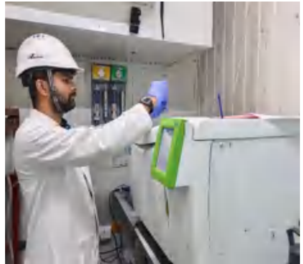
Figure 13: GC-ECD instrument used for PCB analysis
