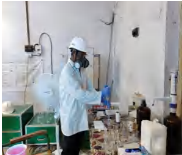
Figure 12: Chemical lab setup for PCB oil extraction
